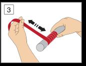
While holding SPITA ResQ-tape in place, begin STRETCHING at 3 to 4 times its length and wrap object with 50% overlap to ensure a proper seal.
